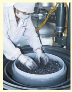
Loading a crucible with feedstock
