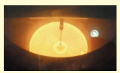
Molten polysilicon inside a monocrystalline furnace
